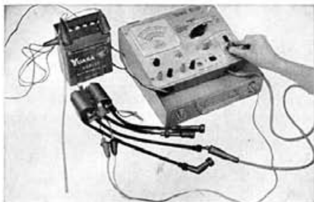
Fig. 7-8 Ignition coil test
