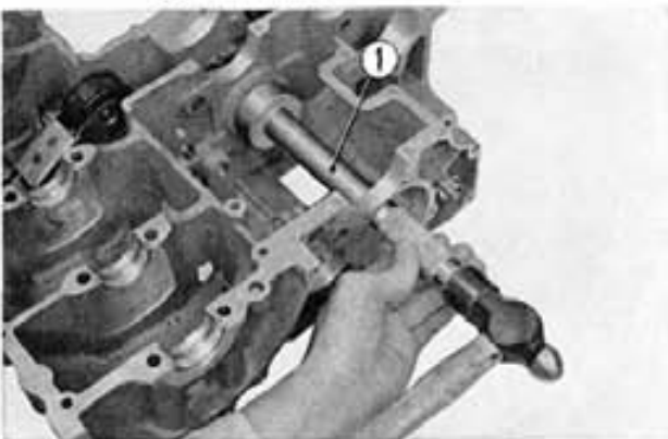
Fig. 5-14 ① Bearing driver tool
