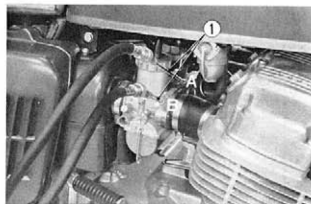
Fig. 6-17 ① Vacuum gauge adapter
